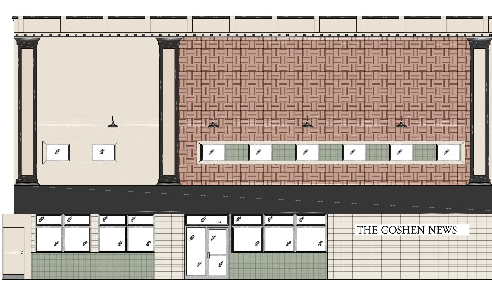
4" TRIM CAP-PRE-FORMED CORNICE-3" EFIS DETAIL BAND-EFIS COLUMN— 3" EFIS DETAIL BAND 4' FULL LENGTH CANOPY (BLACK CLOTH) EXISTING MASONRY-
